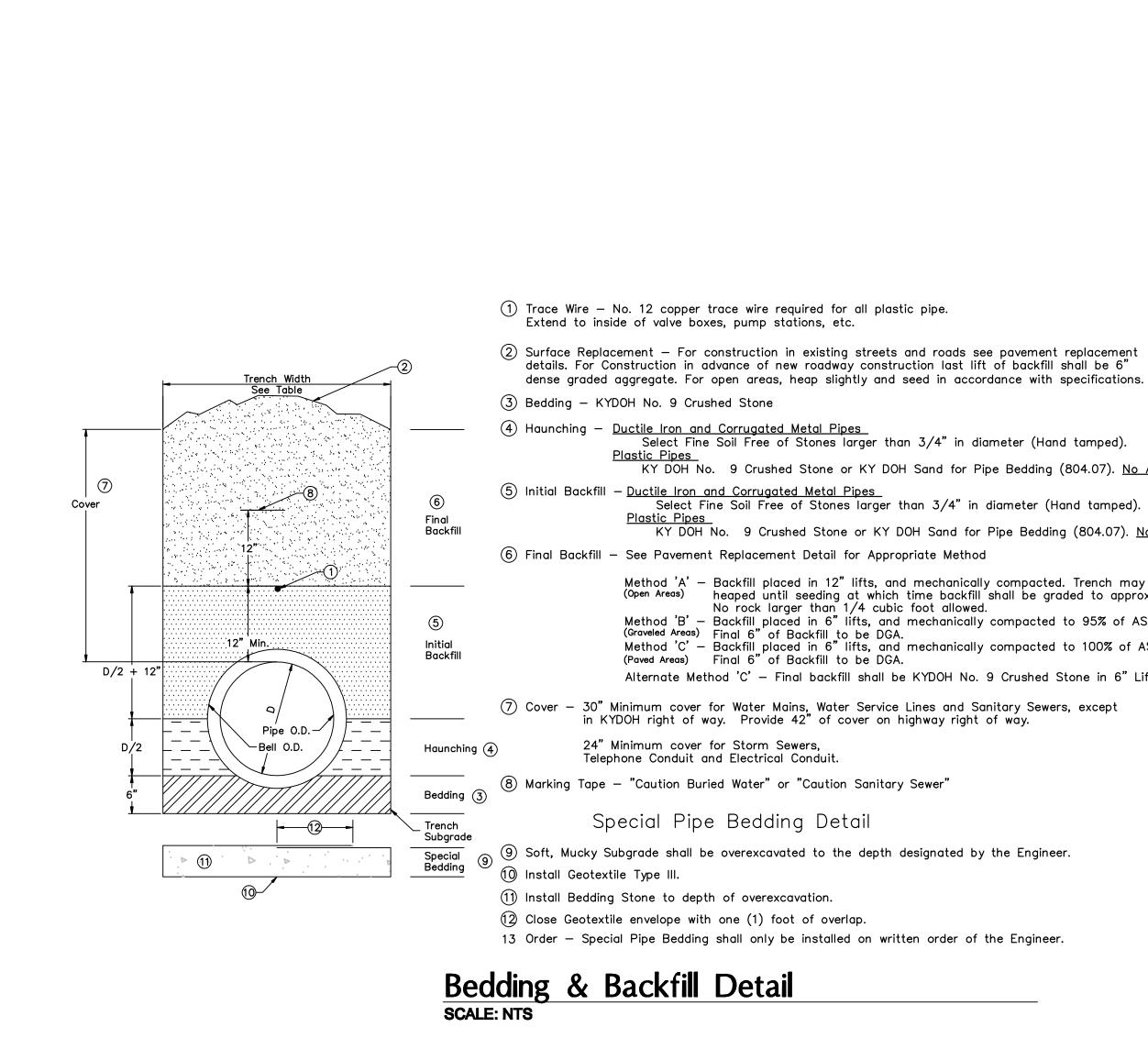
② Surface Replacement - For construction in existing streets and roads see pavement replacement details. For Construction in advance of new roadway construction last lift of backfill shall be 6"
