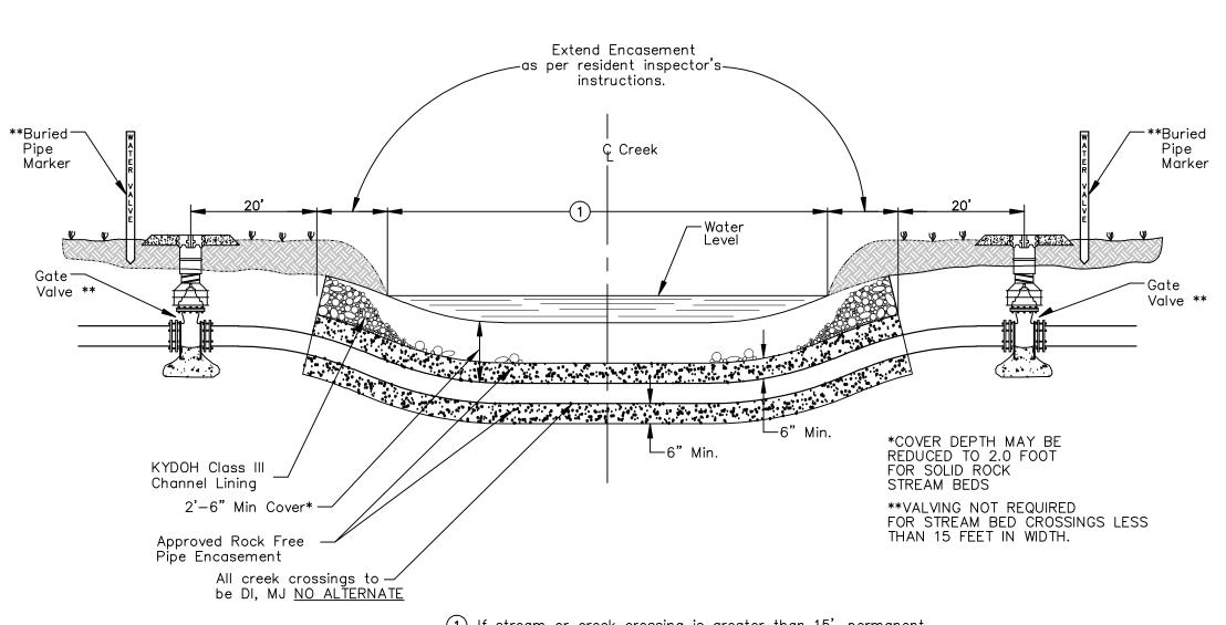
If stream or creek crossing is greater than 15', permanent test points shall be provided on each bank.
